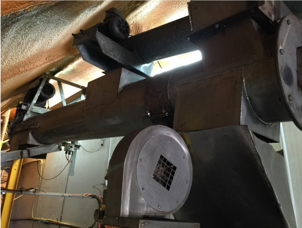
3.6M x 320mm S/S 2 STATION PROCESS AUGER - directional feed gates & head mounted geared motor drives
