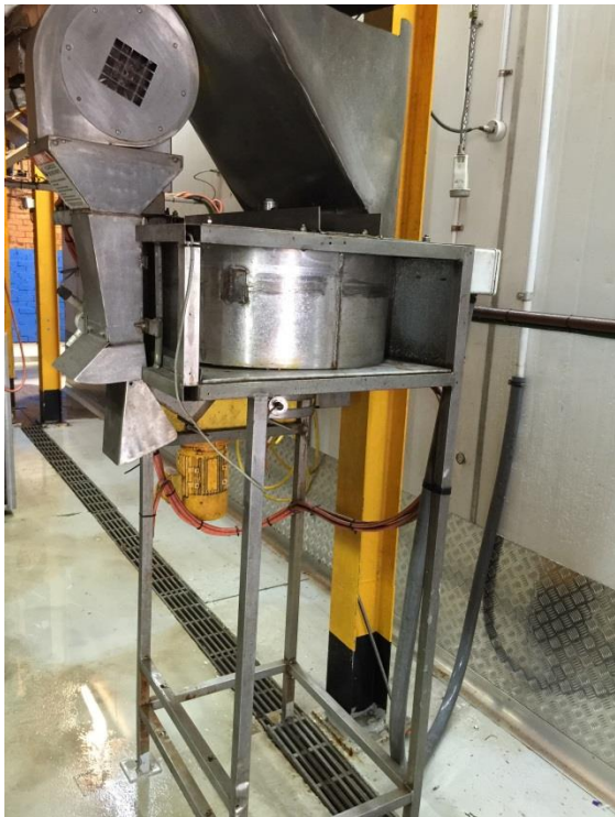
MATHIESON MANUAL ICE BAGGING MACHINE - stainless steel on stand, with top hopper feed & geared motor
