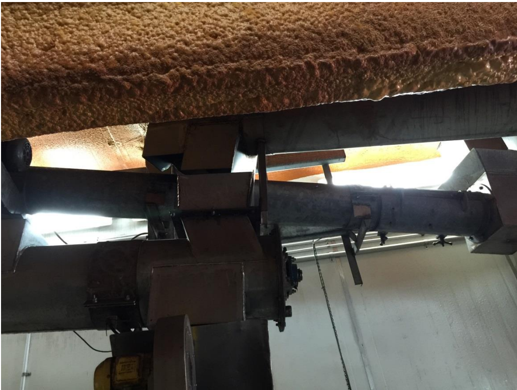
3m x 280mm GAL. AUGER - head mounted geared motor drives
