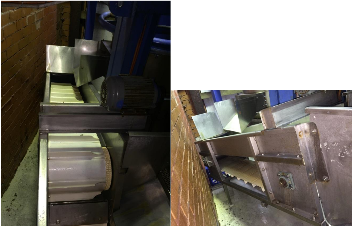
2.2M INCLINE MOTORISED BELT CONVEYOR - Stainless steel frame with cleated belt conveyor, with top mounted geared drive, approx 2200 x 3500mm
