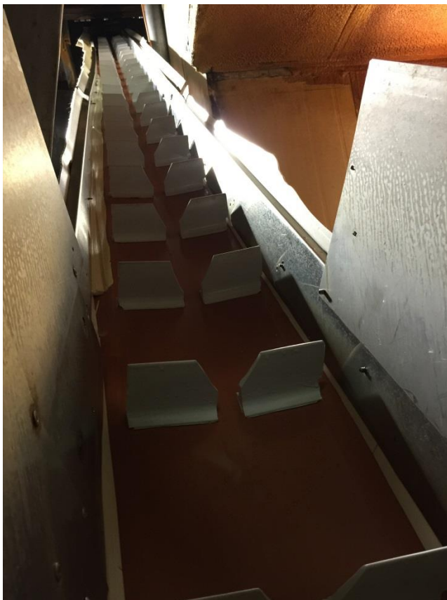
8M MOTORISED INCLINED BELT CONVEYOR - Stainless steel, V-shaped cleated belt with top geared electric motor drive
