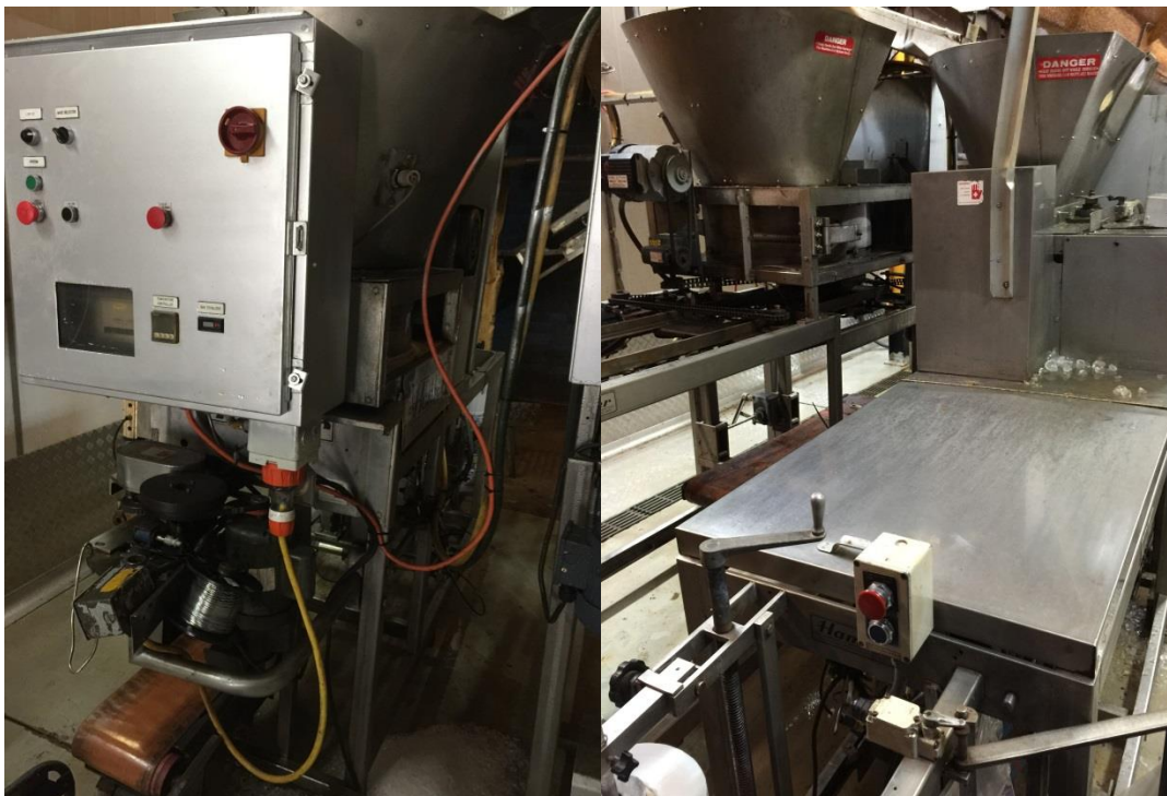
HAMER 310 AUTOMATIC FORM FILL & SEAL MACHINE - 50 bags x 5kg per minute capacity, complete with wire clip tying head model 125, with conveyor bag support & PLC controls
