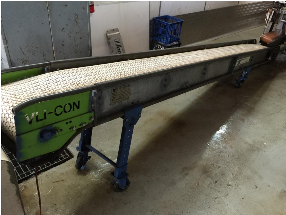
4.4m PIT TOP MOTORISED INCLINED BELT CONVEYOR
