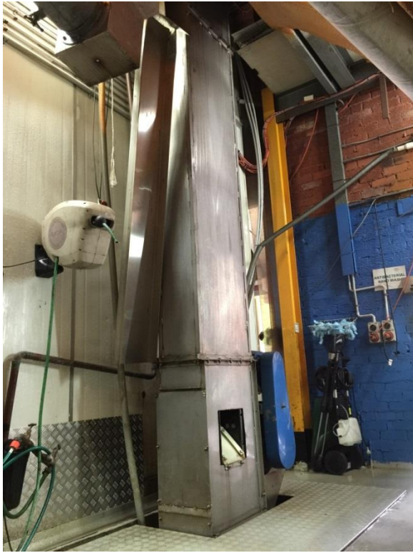
4.5m S/S VERTICAL BUCKET TYPE ICE ELEVATOR - Stainless steel with 2.2kw geared motor drive, approx 4500 x 600 x 300mm
